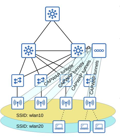
The WLC and lightweight APs use a protocol called CAPWAP (Control And Provisioning Of Wireless Access Points) to communicate.
